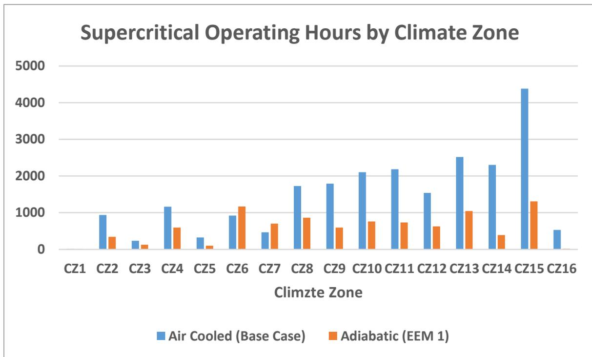
**Figure 7. Supercritical hours (air cooled vs. adiabatic, LSM).**
