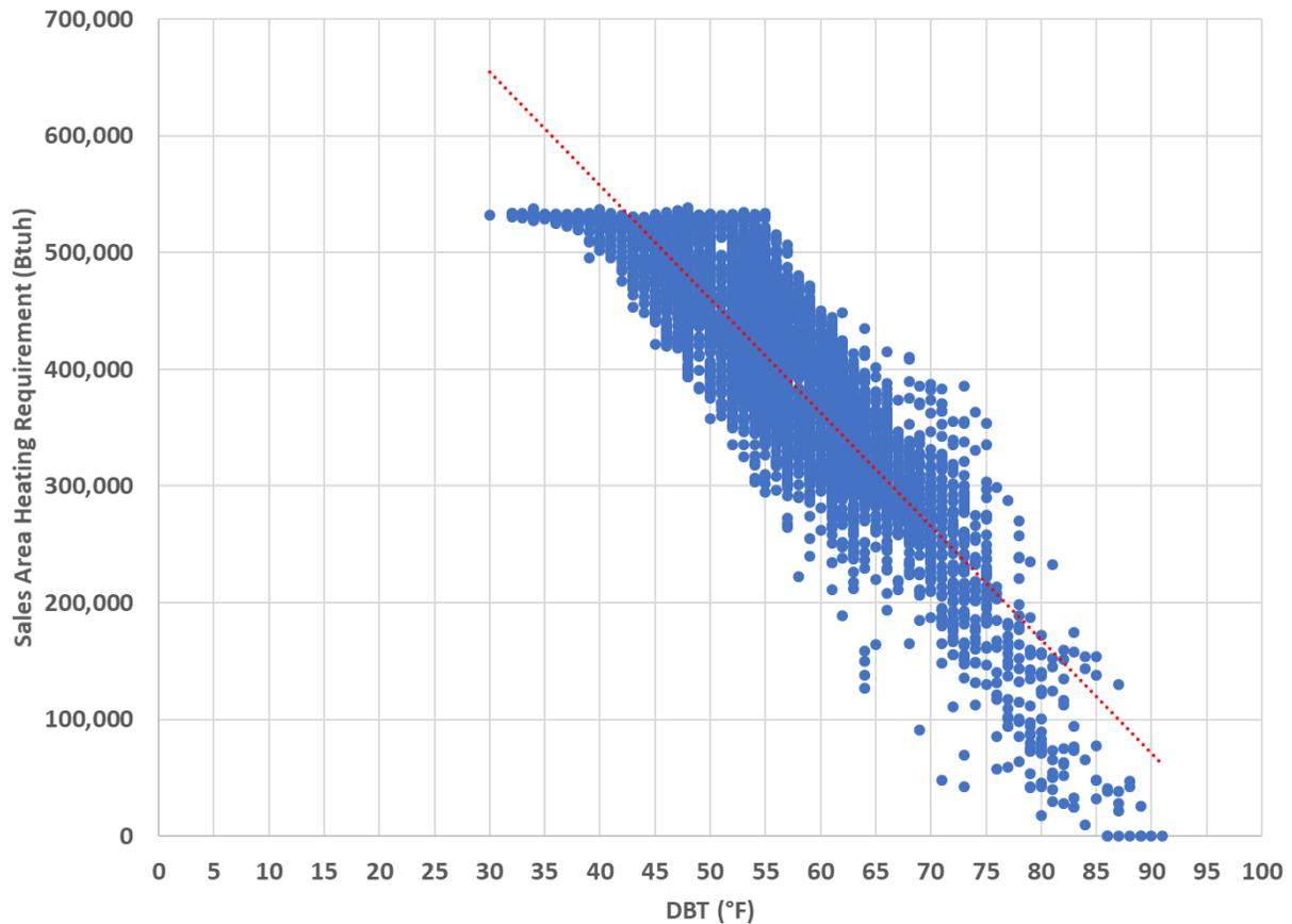
**Figure 4. Balance point temperature for Climate Zone 3.**
