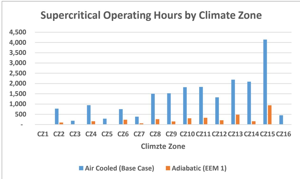
**Figure 6. Supercritical hours (air cooled vs. adiabatic, RWH).**
