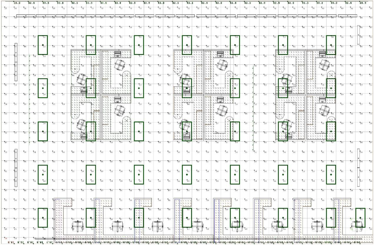
**Figure 52: Plan View 2022 Design B2 (Troffer Lighting Providing Task and General Lighting).**
